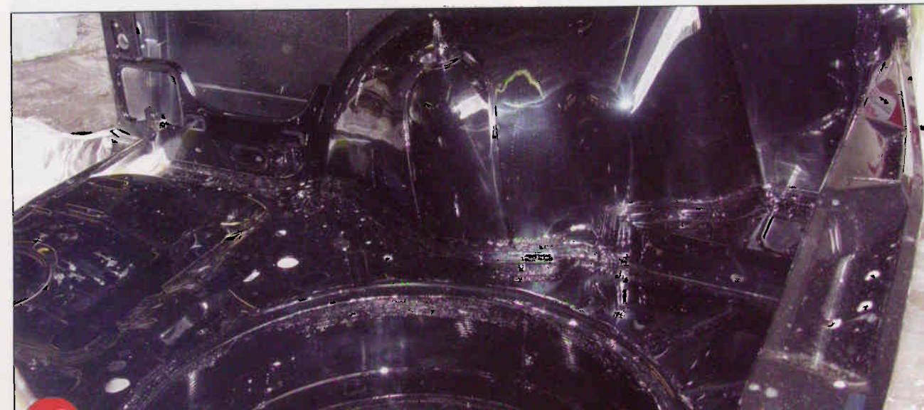
11) The same bare metal treatment was continued over the entire car
