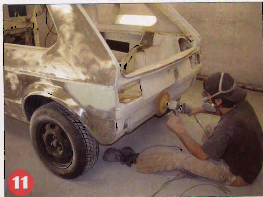
11) The same bare metal treatment was continued over the entire car
