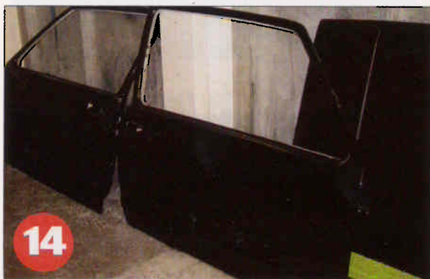
14) The doors and bumpers, hatch and bonnet were all shotblasted off the car before any prep stages and then wet sanded after to a mirror shine
